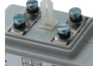
Split output terminals enabling risk-free short-circuiting of the secondary current (M4 or cage for 4 mm<sup>2</sup> wire)
